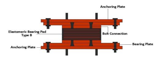
This type of Bearings are Replaceable.
